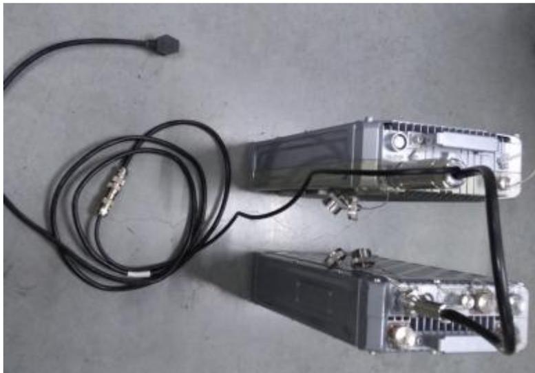
Step 3: Connect feeder and antenna: Connect one end of the antenna feeders (2 pieces) to the RF interface of RRU, connect the other end to the RF antenna. Make sure to tighten them up when connecting, otherwise it may cause the weak signal and lead to failure of registration when the terminal is slightly far away from the system.
