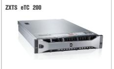
As a control node of voice, data, and trunking services, the CN device ZXTS eTC 200 provides moderate system capacity and throughput and can address the communication needs of education and health systems or small and medium enterprises. It is compact in size and applicable when there is a need for deployment inside a car.
